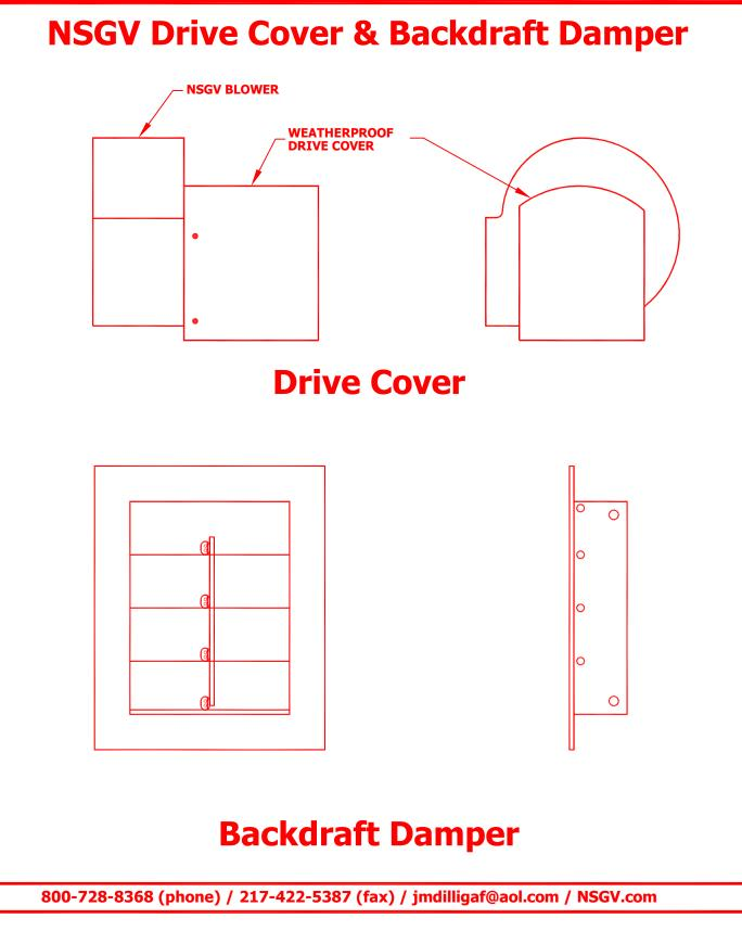
NSGV weatherproof drive covers are constructed from galvanized steel and coated with an air dried enamel paint. Removal of (4) bolts provide total access.
